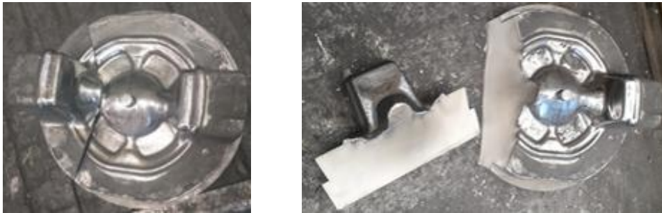
Figure 2. Coated Die situations after the forging process
