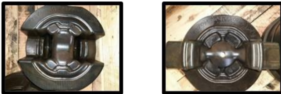
Figure 3. Coated Die situations before the forging process
