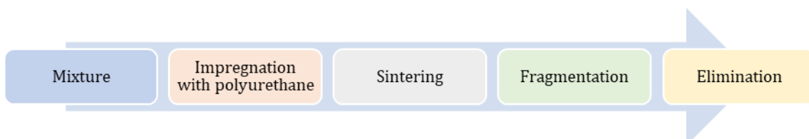
Figure 2. Production technology of Beta Tricalcium Phosphate ( \beta -TCP) with sponge impregnation method [3]
