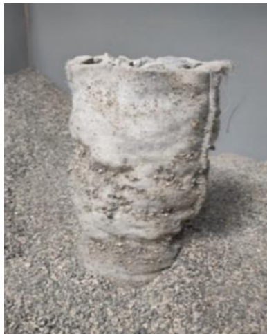
Figure 3. Deformed shape of the geotextile wrapped (G-300) stone column model after loading
