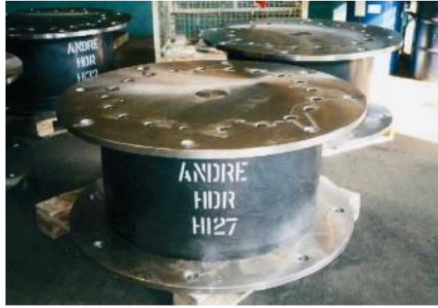
Figure 2. Highly damped rubber insulator
