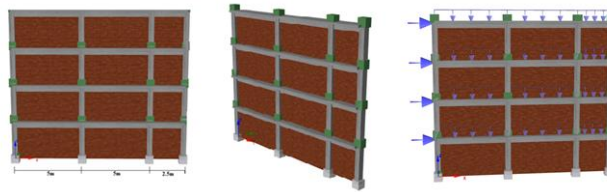
Figure 1. The reference structural model and applied loads
