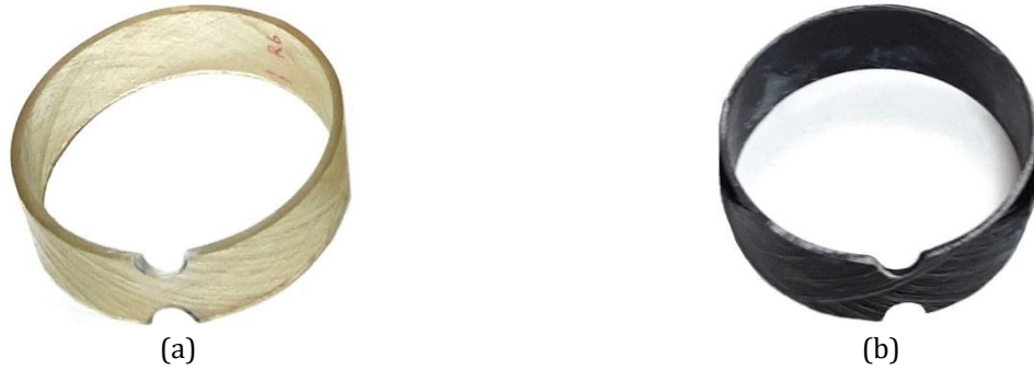
Figure 1. a) Glass fiber/epoxy and b) basalt fiber/epoxy composite samples
